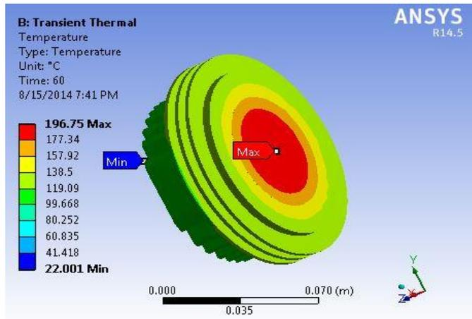
Figure 3: Temperature distribution obtained in the cylinder head at the end of 60 sec
