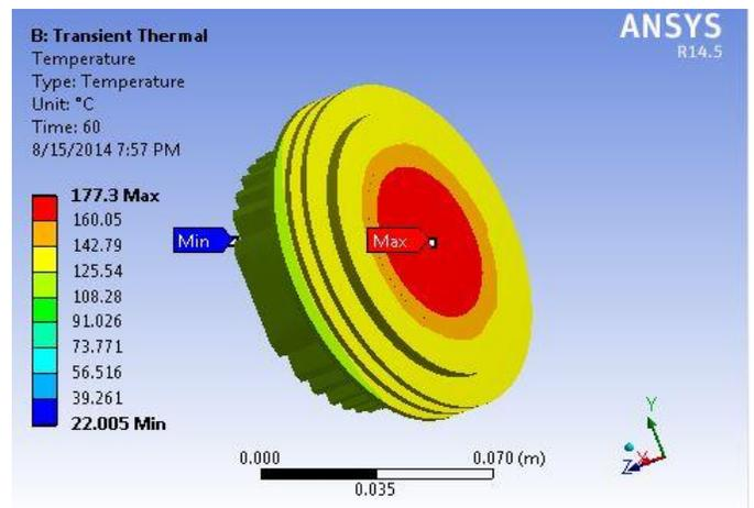
Figure 5: Temperature variation with Time for C443
