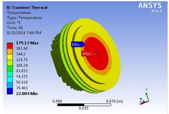
Figure 4: Temperature variation with Time for B390
